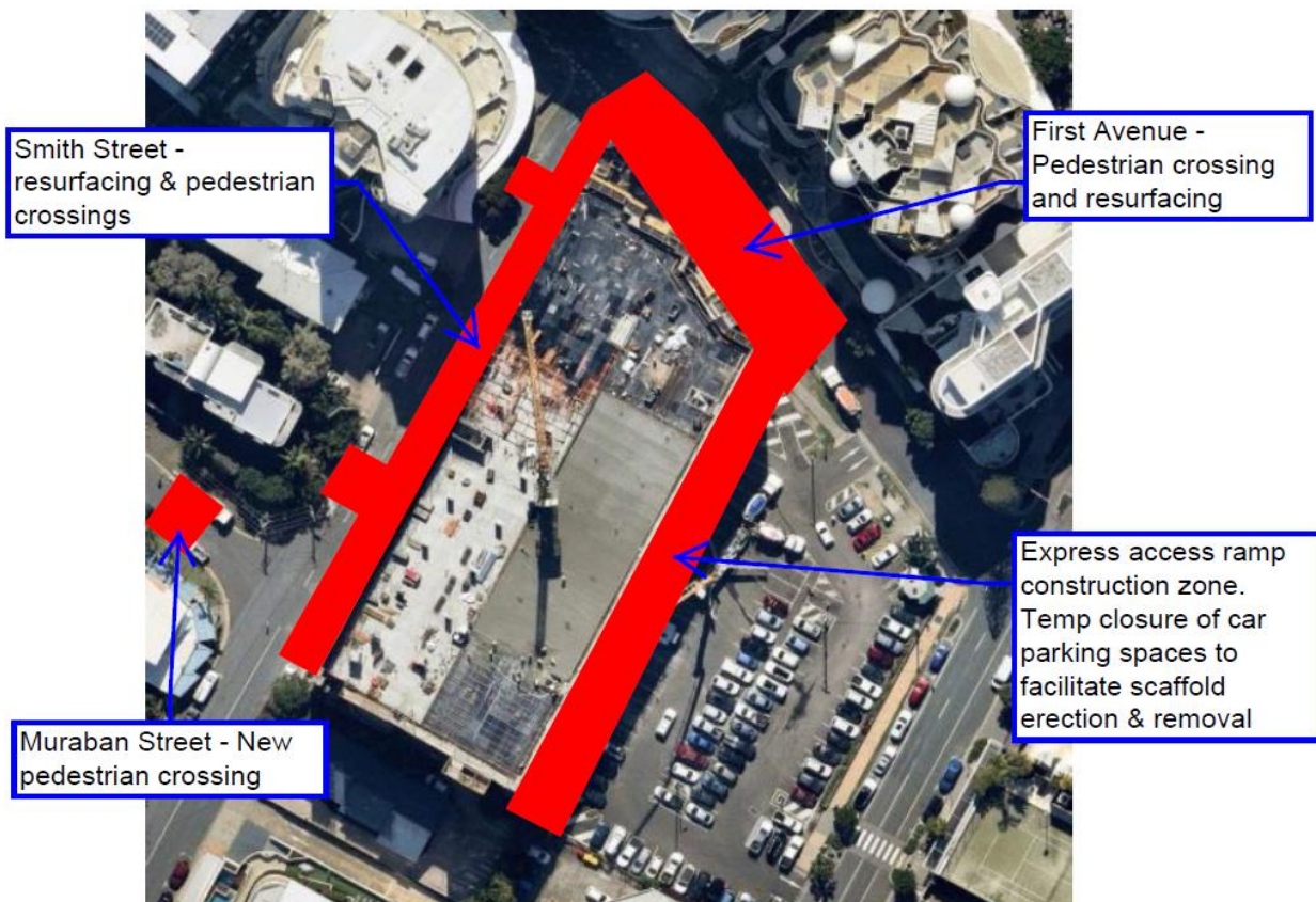
Mooloolaba new multi-deck car park, work areas
